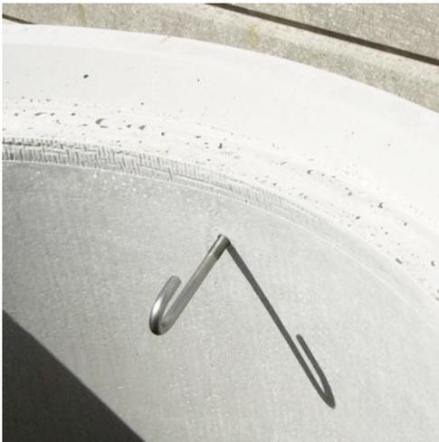
*R264124 Cone vaults are provided with three - 3/8-16 threaded inserts on the inner surface of the cone, 4" below the lid, to be used with stainless steel j-bolts to support splice cases or racking. A pair of threaded inserts is also cast into the inner surface to mount a grounding lug.*
